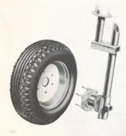
easy-to-change wheels of the Salsbury are an exclusive feature. No disconnecting of brake or chain. Just remove the rim nuts as you would on an automobile and the wheel slips right off the axle. Easy accessibility of all moving parts for service.
