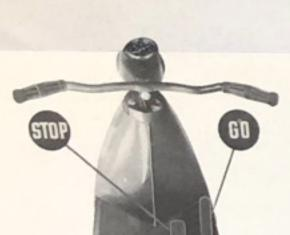
EASIEST TO DRIVE! The Salsbury is the most completely automatic vehicle ever built. Automatic clutch and transmission reduce controls to two pedals—Stop and Go. The Salsbury automatically gears up or down and is the only vehicle made which provides maximum performance for all road conditions.
