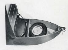
3 BIGGEST PACKAGE COMPART-MENT—one and one-half cubic feet. The Salsbury is the only scooter with a package compartment big enough to carry a spare tire and wheel—and there's room left over for groceries!
