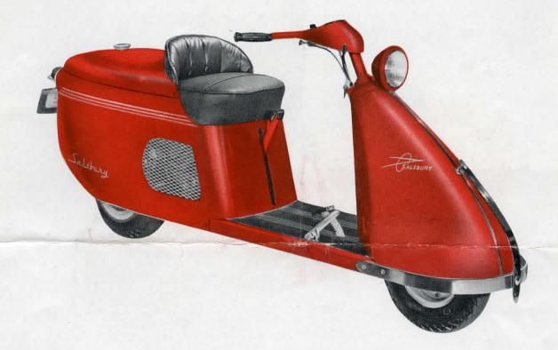
The Salsbury "85" Standard is identical with the De Luxe model except for the front cowling, recessed headlamp and plexiglass windshield. Both models are 88 inches long. Accessory equipment includes side cars, tandem seat, spare tire, speedometer, and frontwheel brake.
