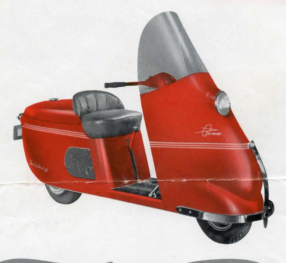
The Salsbury "85" De Luxe comes complete with plexiglass windshield, chromium bumpers, recessed head-lamp, package compartment lock, locking ignition, foot starter, auxiliary hand throttle, choke, protected rear light, leather-covered, inner-spring cushioned seat.
